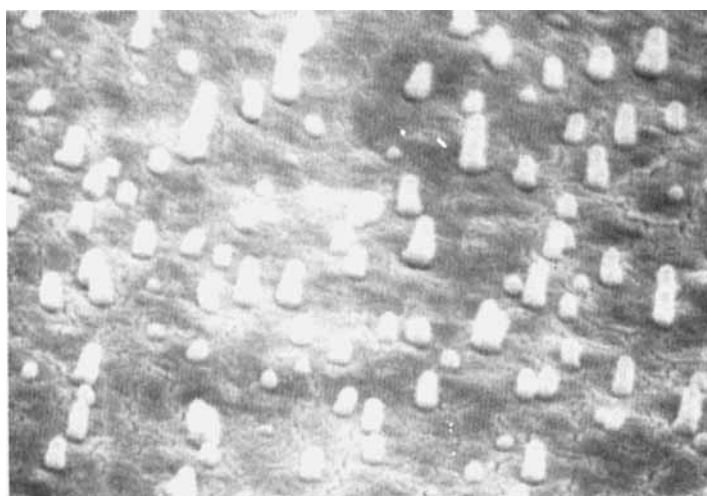
FIGURE 1. Scanning electron micrograph of fractured surface of PBT/HTH10 70/30 blend quenched from the mesophase (original magnification 20000 x).
